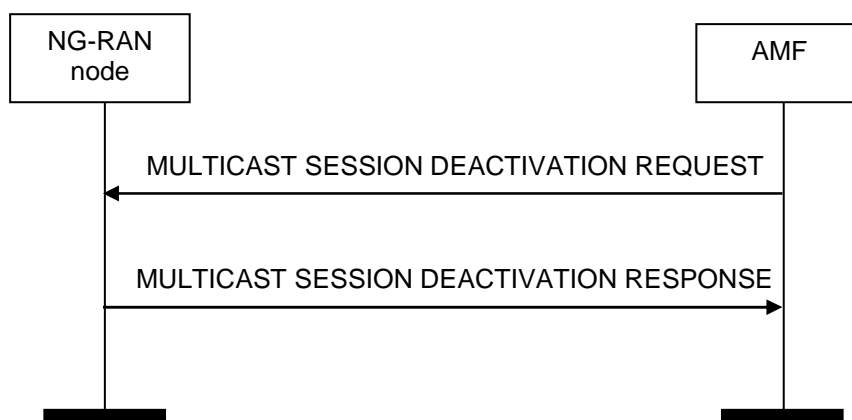
Figure 8.18.4.2-1: Multicast Session Deactivation, successful operation.
