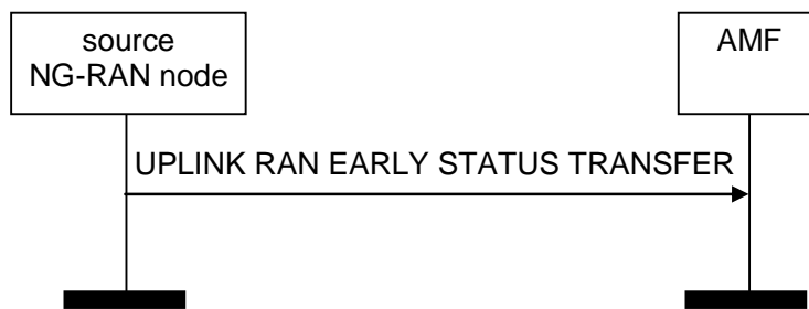
Figure 8.4.9.2-1: Uplink RAN Early Status Transfer
