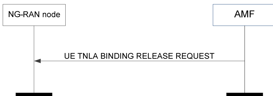
Figure 8.13.1.2-1: UE TNLA binding release request
