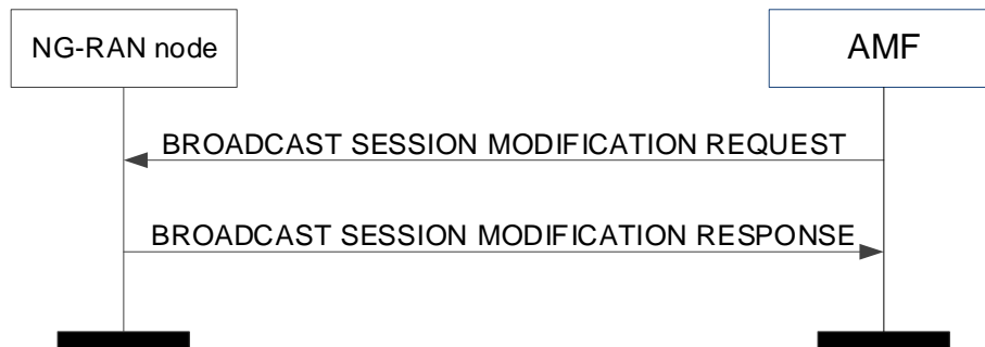
Figure 8.17.2.2-1: Broadcast Session Modification, successful operation.
