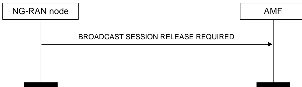
Figure 8.17.4.2-1: Broadcast Session Release Required, successful operation.
