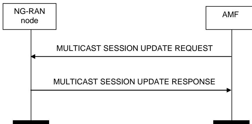
Figure 8.18.5.2-1: Multicast Session Update, successful operation.
