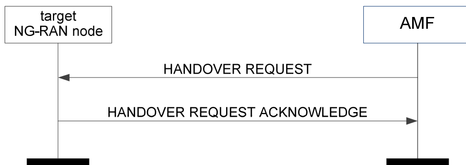
Figure 8.4.2.2-1: Handover resource allocation: successful operation
