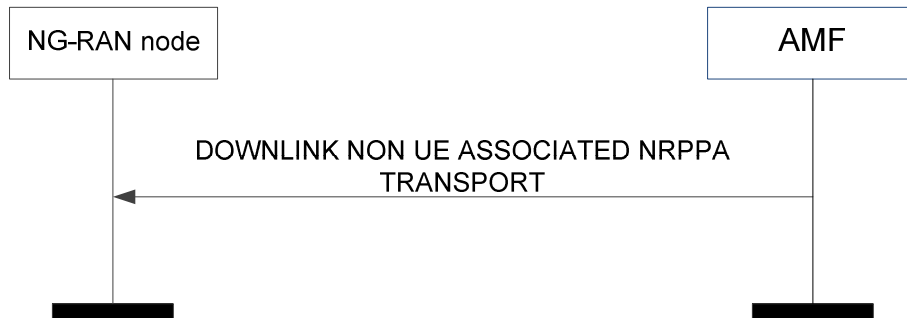
Figure 8.10.2.3-1: Downlink non UE-associated NRPPa transport
